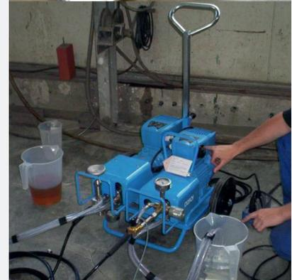
Electric 1 component injection pump
