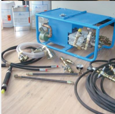
Pneumatic 2 component methacrylate injection pump
